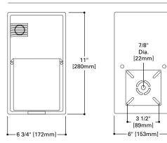
The Lumark WAL-LITE features a injection-molded polycarbonate housing / lens and a die-cast aluminum back plate for rugged durability. U.L. Listed for wet locations. CSA certified.
